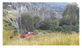
appears that the brake disc had expanded with heat and on cooling down, resumed its normal width resulting in the hand brake pressure being released. Lesson learned here, was to always put a manual car in gear when parking!
